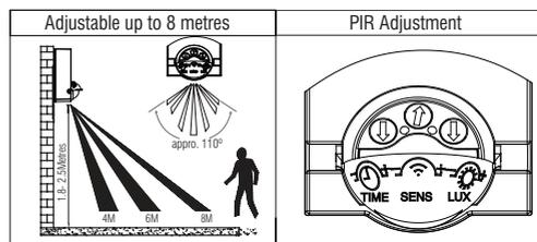
The PIR sensor has a **manual override function** which can be operated by taking the following steps:
