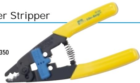
V-notch blades strip a wide range of outer cable jacket. Precision-ground, replaceable knife-type blades strip tight buffer tube insulations (900µm). Also strips mechanically strippable coatings from 250 microns to 900 microns.
