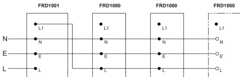
If any of the loads on the circuit are of Class I construction use the earth terminals in the drivers as loop terminals to maintain continuity.
