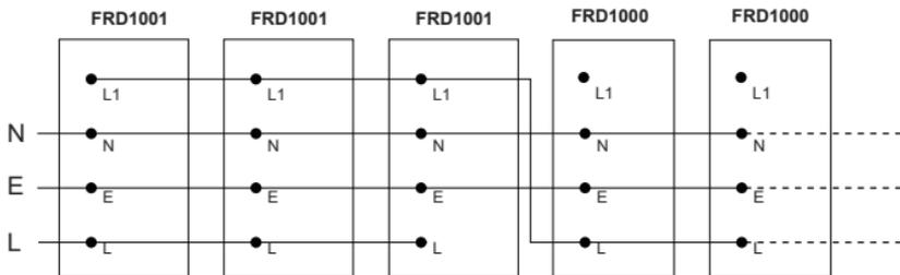
The live, neutral and earth connections from the mains supply must be connected to the nearest FRD1001 at the beginning of the circuit.
