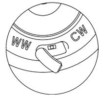
With the Tilt version the CCT Switch is situated on the body of the driver adjacent to the luminaire connecting lead (Fig. 5)
