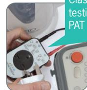
Class 1 PAT testing with the PAT Adapter 1
