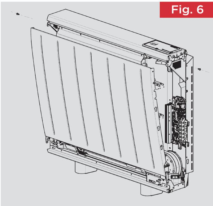
6. Remove the two screws securing the front panel, located at the upper sides of the heater, and swing the upper edge of the front panel upwards and unhook it from along the heater base.
