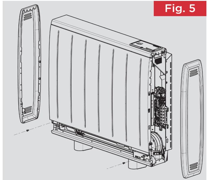
5. Remove the two screws located towards to bottom of either end of the heater, which retain the heater sides.
