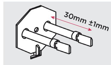
Fit the remaining energy cells to the bottom row, being careful not to damage or dislodge the element.
