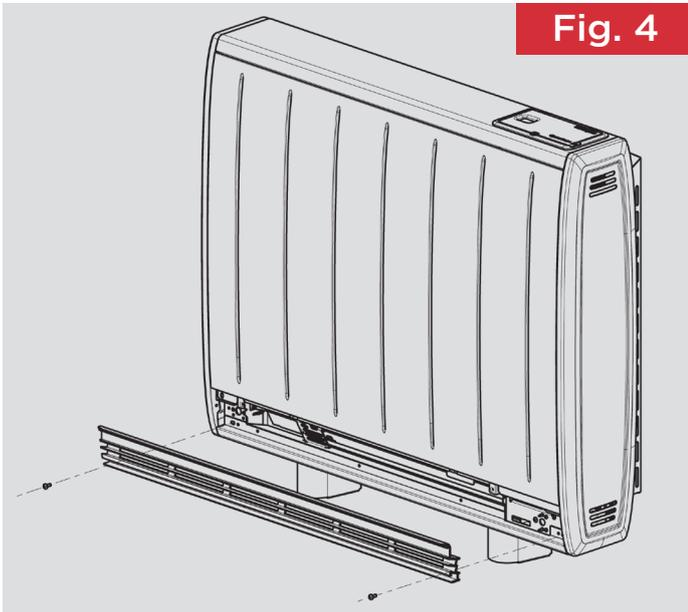
4. Lay the heater on its back before removing the screws which hold the grille panel in position. Set the grille carefully to one side to ensure that it is not damaged.
